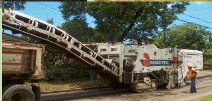
Asphalt Concrete Grinder for recycling existing asphalt concrete
