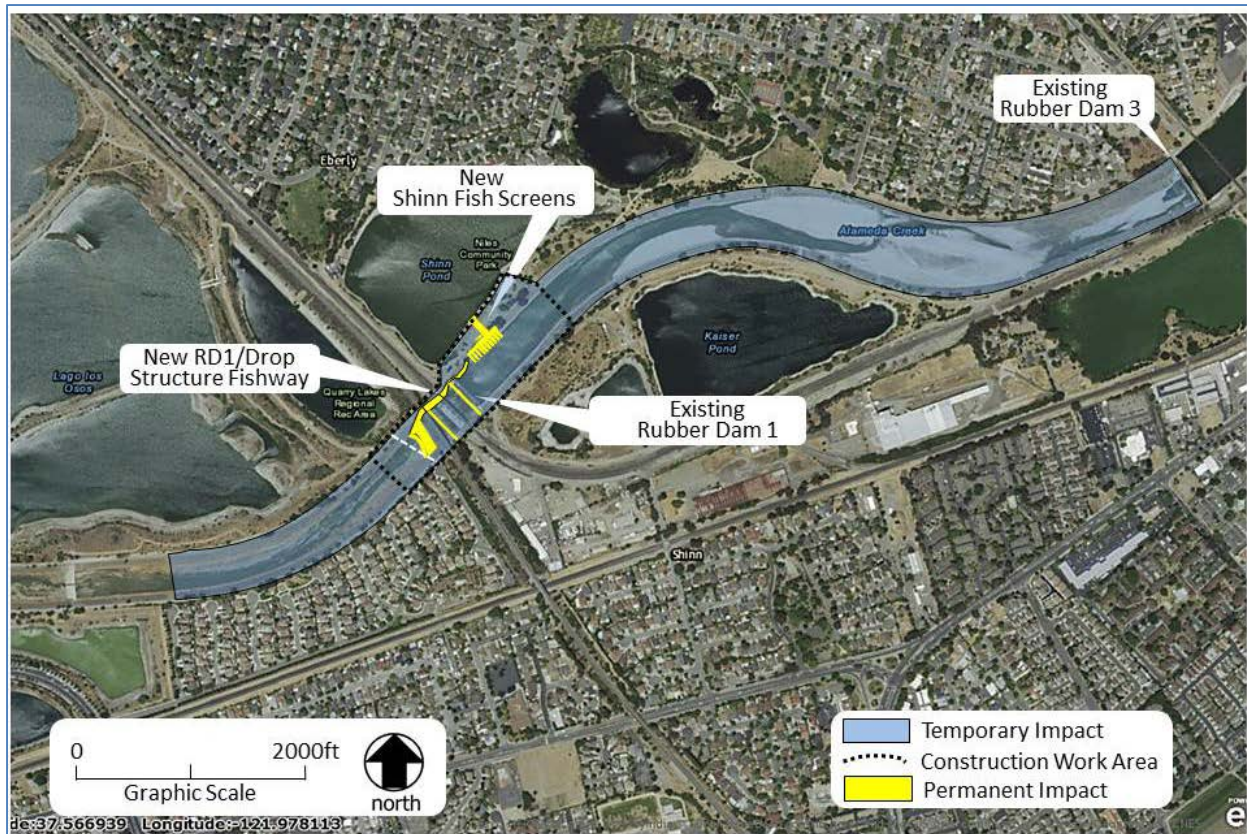
Figure 7. Approximate Locations of RD1/ACFCD Drop Structure Fishway and consolidated Shinn Pond Screens and construction zones.
