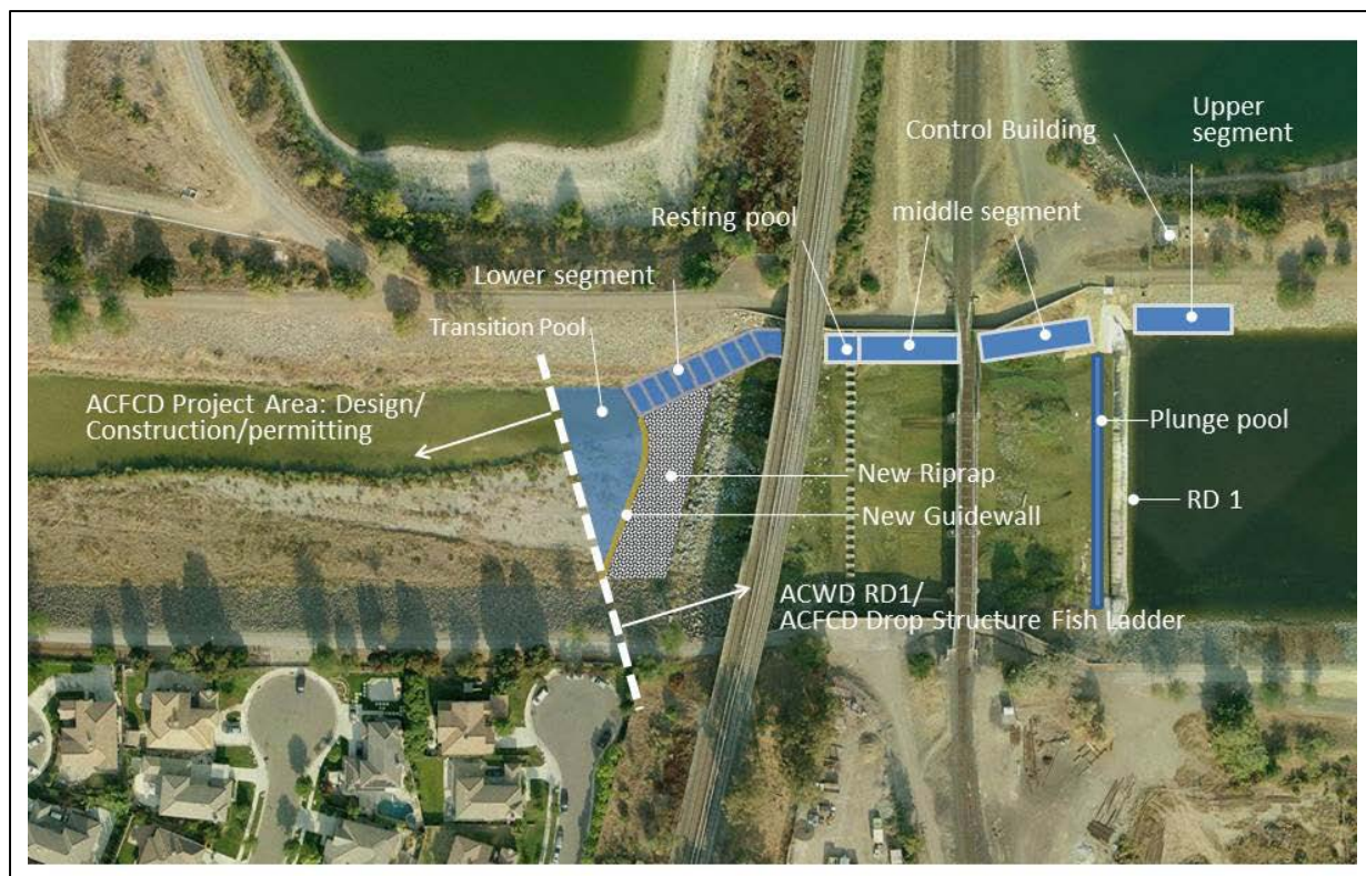
Figure 9. RD1/ACFCD Drop Structure fishway.
