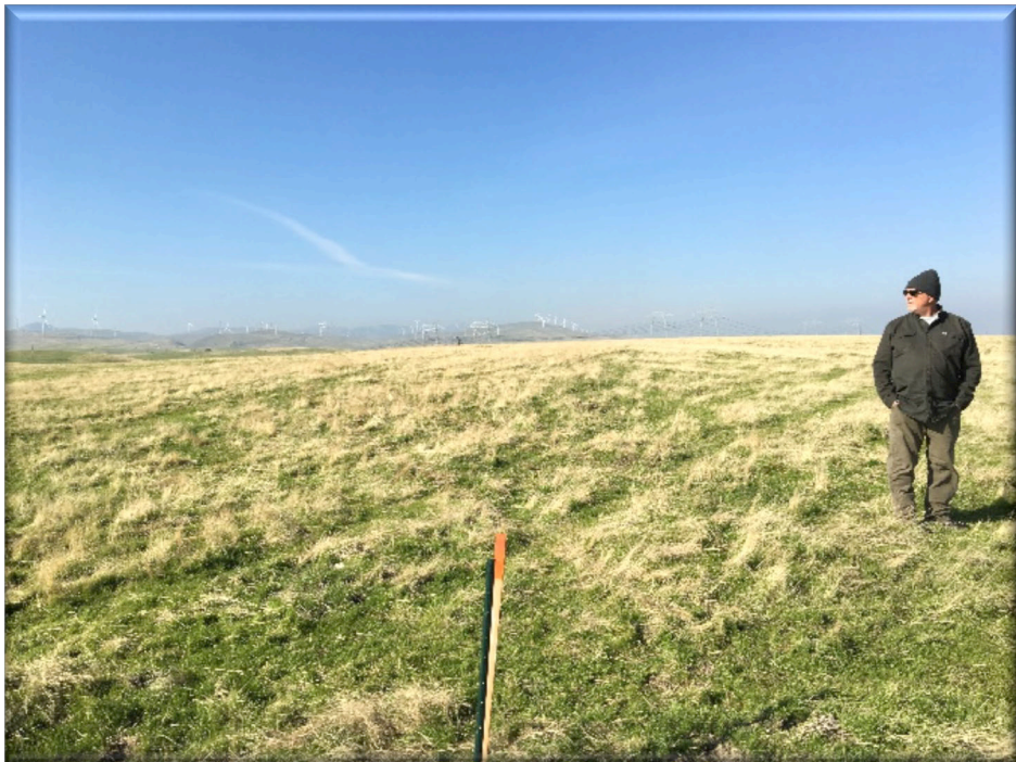
Plate 79. Looking northwest from Site 36A. Recommended location is just up slope from this site. Note that the slope at this location is not extreme, but the turbine pad would create a shallow bench in close proximity to the steeper slope just south of this location.
